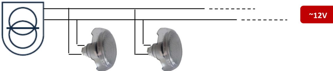
**A N'UTILISER QU'AVEC UN TRANSFORMATEUR ISOLANT DE SECURITE. NE PAS BRANCHER EN SERIE.
